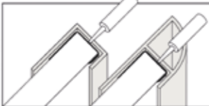
Finishing end trims and Quadrant trims Finishing end trims for panels.
