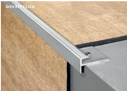
STAIR PROFILE UPPER STEP 200 x 1.5 x 3 cm Use Vinyl Glue to secure the floor vertically to your stairs. The horizontal planks slide into the profile. Compatible with Quick-Step's Vinyl Click ranges.
